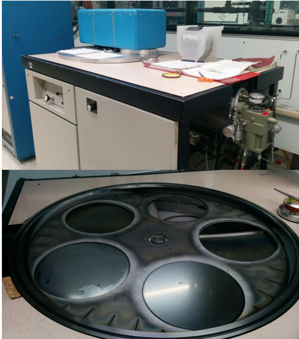
Figure 2.7.1 Top: Overview of the sputter tool. Bottom: Inside view of the sputter tool.
