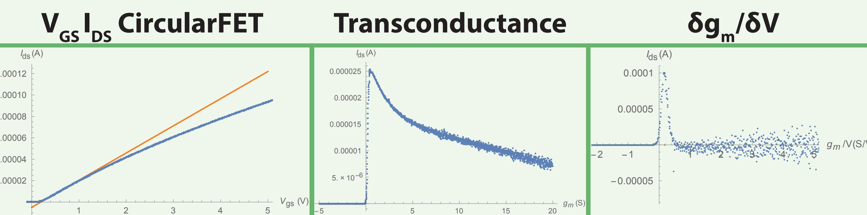
$V_g$  data was used for extracting  $V_{th}$  and  $g_m$ .  $V_{th}$  extraction was done both with fit to max  $g_m$  with extrapolation and with max  $\delta g_m$ . (0.20V vs 0.19V). Mobility and unknown W/L ratios can be found with  $g_m = \mu_n C_{ox} W/L$ .
