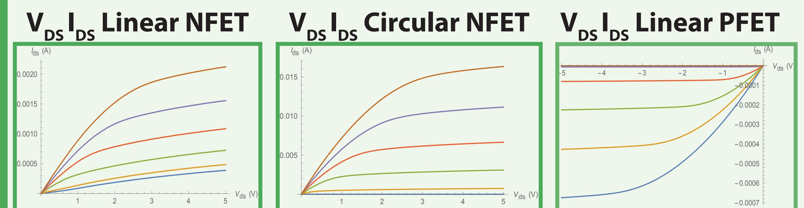
As can be seen in the above graphs, the linear NFET has significantly more leakage current than both the circular PFET and the linear PFET. This is due oxide charge
