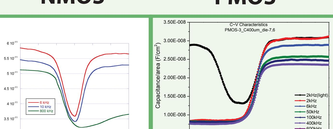
CV curves at different frequencies used to extract device parameters.
